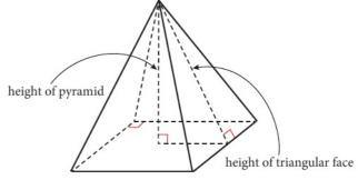
Figure 6.8 Features of a pyramid
