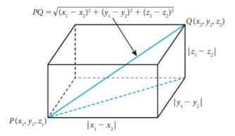
Figure 6.6 The distance between two points in space
