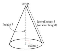
Figure 6.7 Features of a cone
