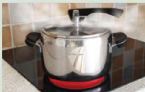
Figure 6.1.7 A pressure cooker cooks foods at pressures above atmospheric pressure and the resulting higher boiling temperature of the water inside decreases cooking time considerably.
