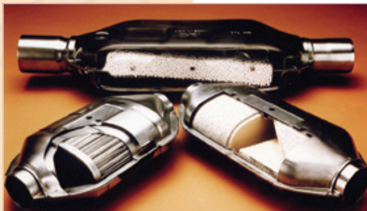
Figure 3.2.9 A variety of catalytic converters are used in car exhaust systems.
