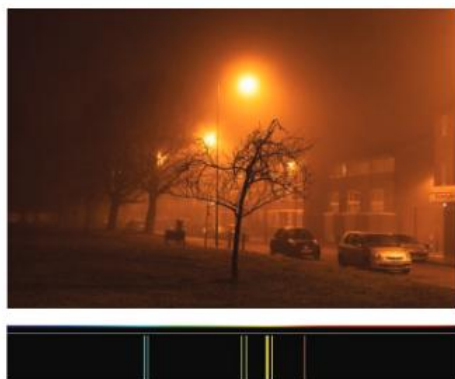
▲ Figure 2.2.1. A sodium lamp and its emission spectrum
