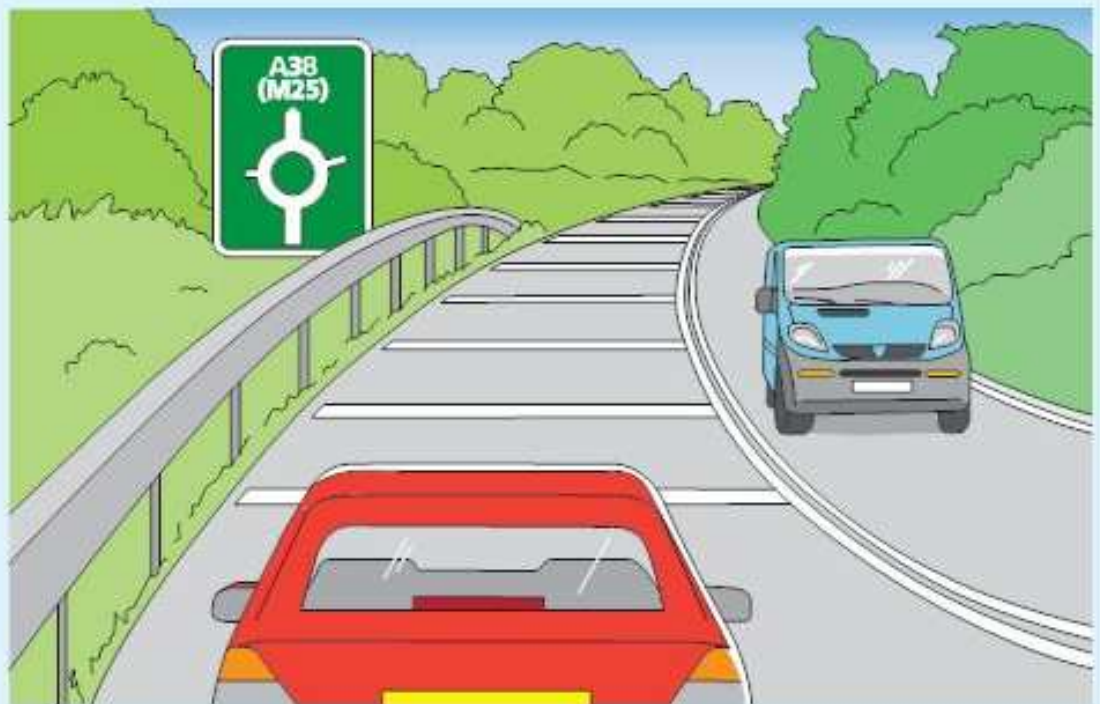
■ Figure 2.10 Road markings giving a false impression of speed to slow drivers down
